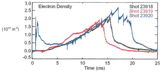
FIG. 4 (color). Interferometer measurement of electron density for three discharges shown in Fig. 3. These measurements have an error of  $\pm 1 \times 10^{18}$  electrons/m<sup>3</sup>.
