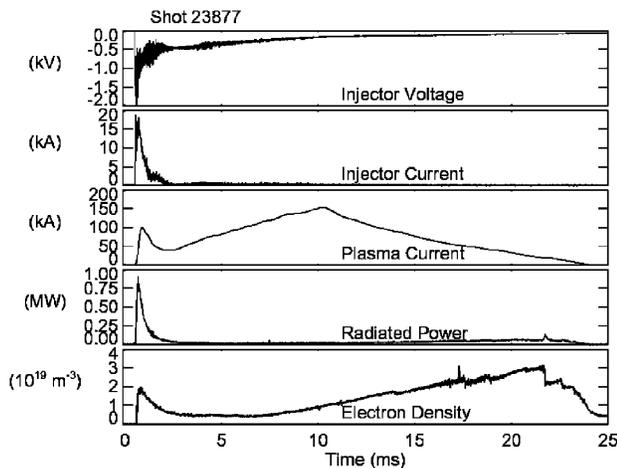
FIG. 2. CHI startup using half-swing of the central transformer. After the CHI discharge is produced, induction is applied at 1.2 ms. The top trace shows the applied injector voltage. The bottom trace shows interferometer measured electron density at the device midplane. The uncertainties on the injector voltage, injector current, and divertor flux are less than a few percent.
