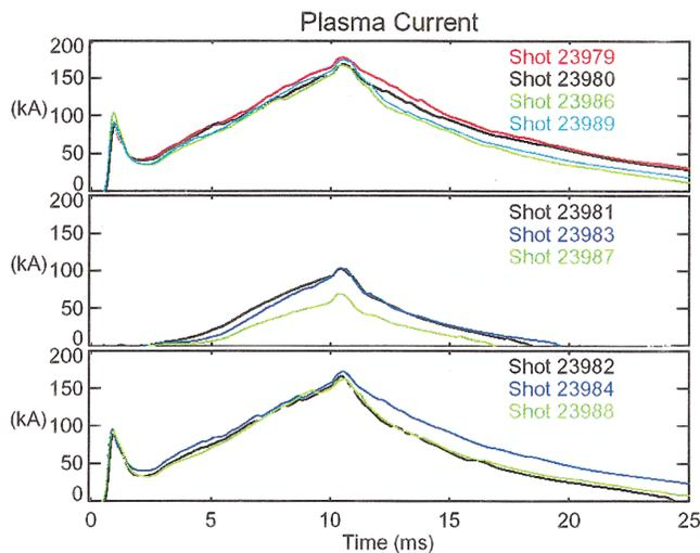
FIG. 5 (color). Comparison of discharges with the same magnetic flux configuration and with vertical field along the outer wall, and operated with and without the application of CHI voltage startup. In shot Nos. 23981, 23983, and 23987, no CHI voltage was applied. For shot No. 23988 the applied CHI voltage of 2.5 kV was above the threshold voltage of 2.4 kV used for the rest of the shots with CHI startup. The inductive voltage history is the same as that for the shot sequence in Fig. 3.
