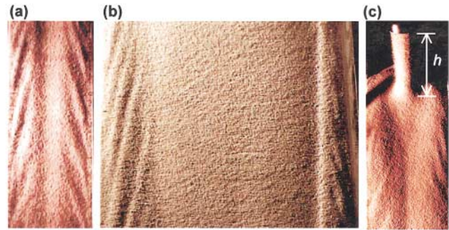
FIG. 3 (color). Varying chute width (a) 7.6 cm and (b) 20.4 cm. (c) Grain impingement zone for 7.6 cm chute. In all cases, \theta = 25^\circ , h = 6 cm, and mass flow = 281 \pm 2 g/s.
