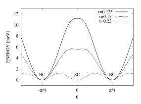
FIG. 4. Mean-field energy per stripe cell (eight Cu's) as a function of the collective phase  $\theta$  of the CDW for various doping levels and for d = 4 stripes in a  $4d \times 12$  system.
