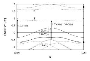
FIG. 2. Electron mean-field bands measured from the chemical potential for the momentum in the direction of the stripe (d = 7, x = 0.071). The arrows are the lowest energy dipole allowed mean-field transitions in a  $d \times 4$  cluster, labeled by energy and polarization. The x polarization is perpendicular to the stripe. The full dots indicate the insulating charge transfer gap.
