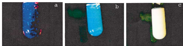
FIG. 2 (color). Color pictures of the PNIPAM microgel dispersion with polymer concentration of 16.9 g/L at various temperatures: (a) 21 °C, (b) 26 °C, and (c) 35 °C. The average hydrodynamic radius of PNIPAM microgel spheres in water at T = 25 °C is 133 nm. The diameter of the vial is 1 cm.
