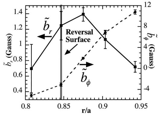
FIG. 3. Radial profile of radial (—■—) and toroidal (---◆---) magnetic-field fluctuation amplitudes at the reversal surface for the resonant,  $n = -1$ , toroidal mode during sawtooth crashes.
