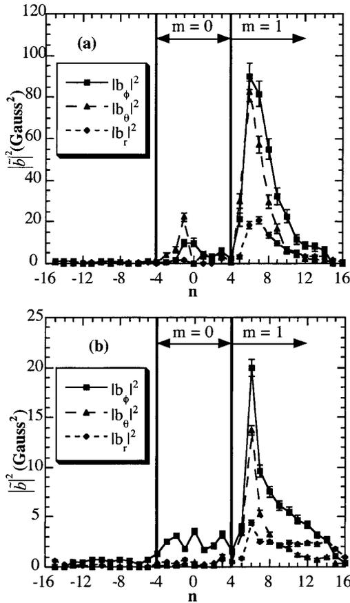
FIG. 2. Toroidal mode spectra of radial, poloidal, and toroidal magnetic fluctuation power at the reversal surface ( $r/a = 0.846$ ): (a) during sawtooth crashes and (b) between sawtooth crashes.
