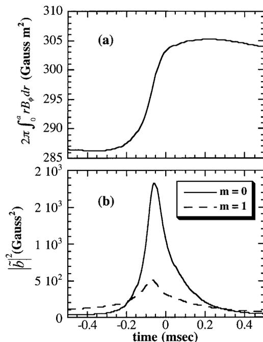
FIG. 1. (a) Toroidal magnetic flux vs time during a sawtooth crash. The time  $t = 0$  denotes the end of the sawtooth crash time (time of maximum time rate of change of the flux). (b) Total magnetic-field fluctuation power in  $m = 0$  and  $m = 1$  poloidal modes at the plasma surface during sawtooth crashes.
