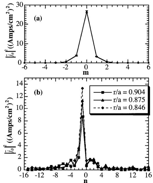
FIG. 4. (a) Two-point poloidal mode number spectrum and (b) toroidal mode number spectrum of poloidal current density fluctuations at the reversal surface during sawtooth crashes.
