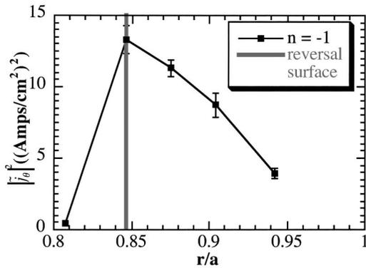
FIG. 5. Radial profile of poloidal current density fluctuation power for the reversal surface resonant,  $n = -1$ , toroidal mode during sawtooth crashes.
