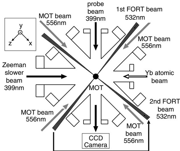
FIG. 1. Top view of the typical experimental setup of a crossed FORT which consists of two right-angled beams. Two counterpropagating MOT beams perpendicular to this paper are omitted in this figure. This setup is referred to as setup I in the text.
