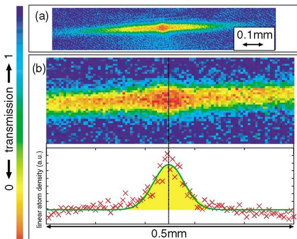
FIG. 2 (color). (a) Typical absorption image signal of the  $^{174}\text{Yb}$  atoms trapped in the crossed FORT. (b) Enlarged signal of (a) near the cross region and the column density profile which was directly obtained from the absorption images. The green line showed the fitting line with the function  $a_1 + a_2 \exp[-(x^2/x_0^2)]$ . The atom number in the cross region (yellow region) was referred to as the  $N_c$  in the text.
