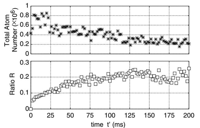
FIG. 3. Time evolution of the total atom number  $N_t$  (asterisks) and the ratio  $R$  (open squares) after a time  $t'$  from suddenly turning on the second FORT at  $t' = 0$  (sudden deformation).
