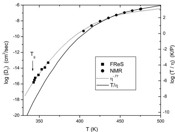
FIG. 2. Comparison of the temperature dependence of translational diffusion with the viscosity.  $D_T$  for TNB determined from FReS and NMR [11] is given on the left axis. Temperature over viscosity [6] is given by the solid line, with scale on the right-hand axis, shifted in order to permit overlap of the high temperature values of the viscosity and  $D_T$  values. The dashed line is  $\eta^{-0.77}$ , vertically shifted.
