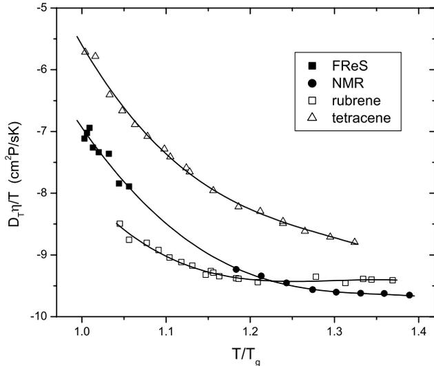
FIG. 3.  $D_T$  from FReS and NMR [11] multiplied by  $\eta/T$ . Translational diffusion measurements of the probes rubrene and tetracene in TNB [3] are also shown. The significant temperature dependence of  $D_T \eta/T$  is inconsistent with the Stokes-Einstein equation and provides evidence for the spatially heterogeneous description of dynamics in the supercooled regime. Solid lines are guides to the eye.
