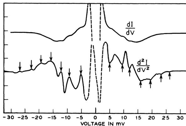
FIG. 1. First and second differentiation of the current through an Al-Al<sub>2</sub>O<sub>3</sub>-superconducting Pb sandwich as a function of bias. (Because of the instrumentation involved, the second derivative trace appears upside down.)
