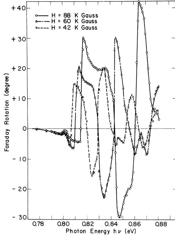
FIG. 2. The Faraday rotation in the second Ge sample for strong magnetic fields at room temperature. The field was applied in [110] direction.
