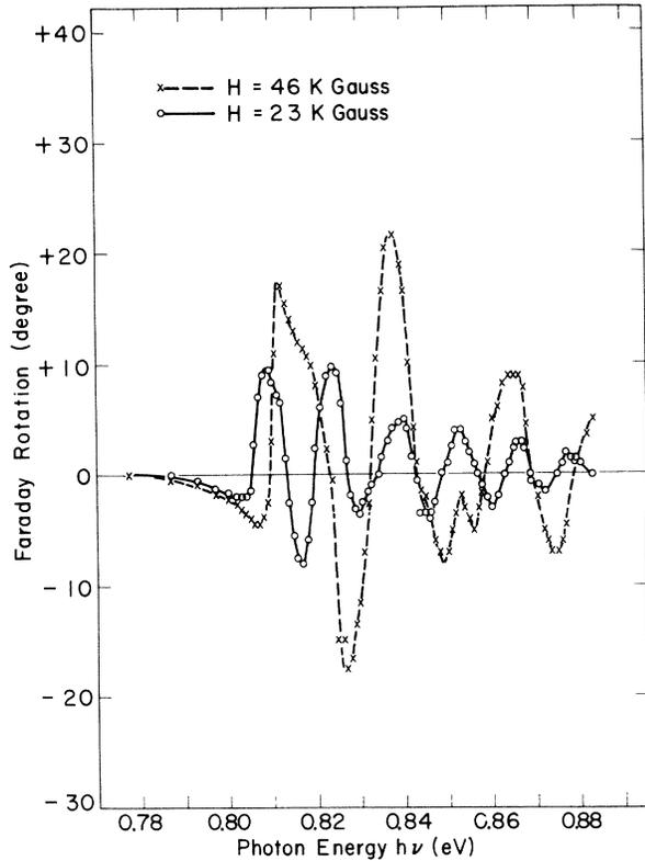
FIG. 1. The Faraday rotation in a Ge single crystal for weak magnetic fields as functions of incident photon energy at room temperature. The field was applied in [110] direction.
