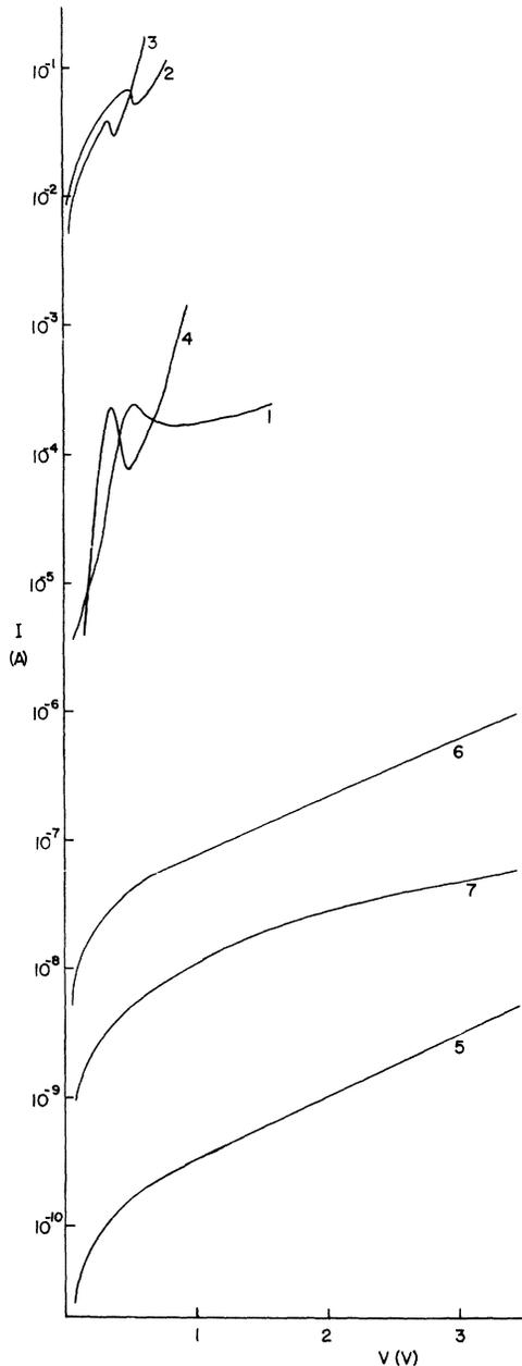
FIG. 2. Curve 1: Pt/Cu with 100Å crystal. Curve 2: Mo/Cu with 100Å crystal. Curve 3: W/Cu with 100Å crystal. Curve 4: Mo/Cu with 300-400Å crystal. Curve 5: Pt/Cu with stacked layers of crystals. Curve 6: Pt/Cu with nitrocellulose film. Curve 7: Pt/Cu with electron-irradiated polyethylene crystal.
