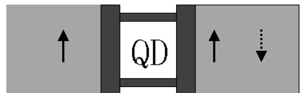
FIG. 1. Schematic plot of the F -QD- F system considered in this work.
