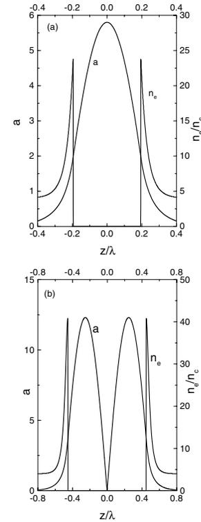
FIG. 1. Analytical solutions of the EM wave amplitude  $a$  and electron density  $n_e$  as a function of space  $z/\lambda$ , for the soliton model with background ion density  $n_i/n_c = 4$ : (a) single hump solution, (b) double hump solution.
