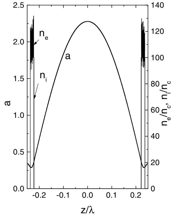
FIG. 3. PIC simulation of the evolution of the laser-plasma interaction. Snapshots of the laser field  $a$ , electron density  $n_e$ , and ion density  $n_i$  after 9 laser cycles. The pump laser amplitude rises from zero to  $a = 0.5$  in three laser cycles and then remains constant. The gap width is  $\Delta/\lambda = 0.443$ . The electron layers are the same as in Fig. 2.
