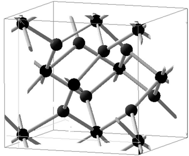
FIG. 1. Si-epitaxial  $\text{ZrO}_2$ . Grey (black) atoms: O (Zr).
