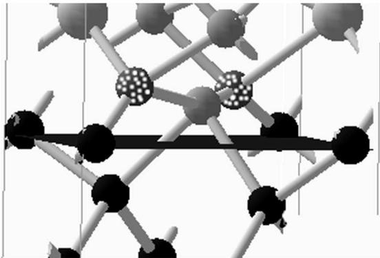
FIG. 2. The [mixed metal-Si]/[O 50% vacant] interface (black: Si; grey: metal; white-dotted: O).
