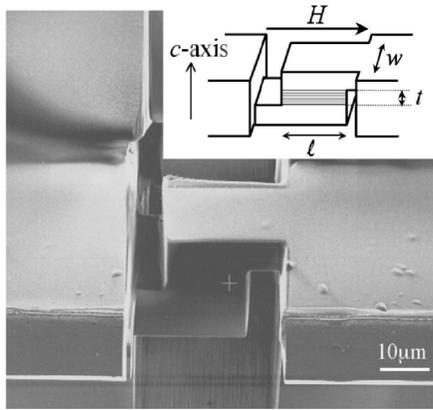
FIG. 1. An FIB image of a typical sample. Schematic drawing of the junction (hatched part) is shown in the inset. The magnetic field is applied along the  $l$  direction. A definition of the junction dimensions is also indicated.
