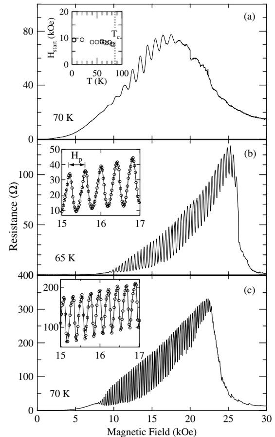
FIG. 2. Flow resistance of Josephson vortices as a function of magnetic field of samples A (a), B (b), and C (c) with an applied current of 1, 1, and  $10 \mu\text{A}$ , respectively. The inset of (a) shows the temperature dependence of  $H_{\text{start}}$  for sample B. The enlarged figures of the flow-resistance oscillations of samples B and C are shown in the insets of (b) and (c), respectively.
