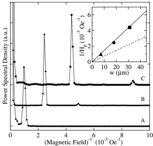
FIG. 4. Power spectral densities of the oscillations for samples  $A$ ,  $B$ , and  $C$ . The vertical axes are shifted properly. In the inset, solid markers show the inverse of  $H_p$ , which is estimated from the positions of the peaks in the spectra, as a function of the sample width ( $w$ ). The broken and solid lines represent  $1/H_0(w)$  and its double, respectively.
