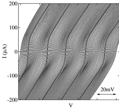
FIG. 3.  $I$ - $V$  characteristics of sample  $B$  at various fields from 14 k to 16 kOe for every 20 Oe at 65 K. Each curve is shifted by a 1 mV step. Bold lines show  $I$ - $V$  curves where the resistance is minimum.
