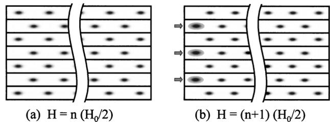
FIG. 5. Schematic pictures of the configuration of Josephson-vortex lattice when the magnetic fields are equal to (a)  $n(H_0/2)$  and (b)  $(n + 1)(H_0/2)$ , where  $n$  is an integer.
