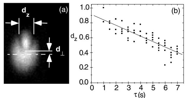
FIG. 2. (a) Schematic of the extraction of  $d_z$  and  $d_{\perp}$  from the vortex line. (b) Evolution of  $d_z$  with  $\tau$ . Each point corresponds to a single image.
