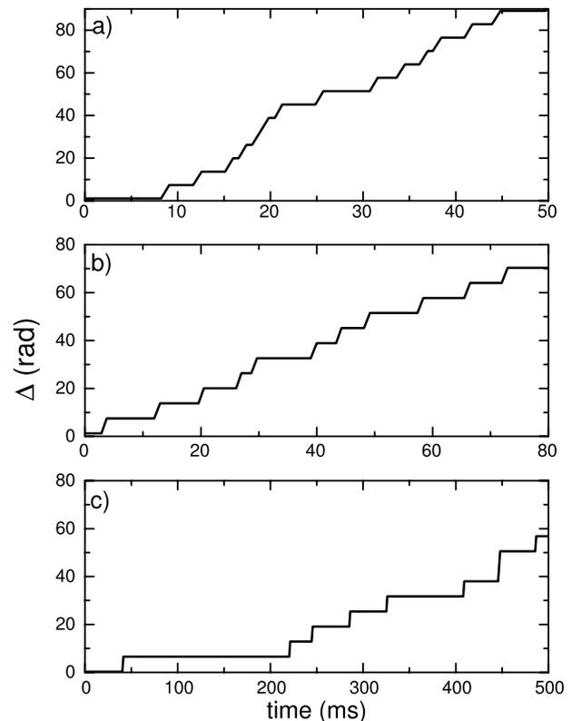
FIG. 2. Temporal evolution of  $\Delta \equiv |\phi_e - \phi_s|$  for (a)  $\nu = 2.05$  kHz, (b)  $\nu = 1.85$  kHz, and (c)  $\nu = 1.70$  kHz.
