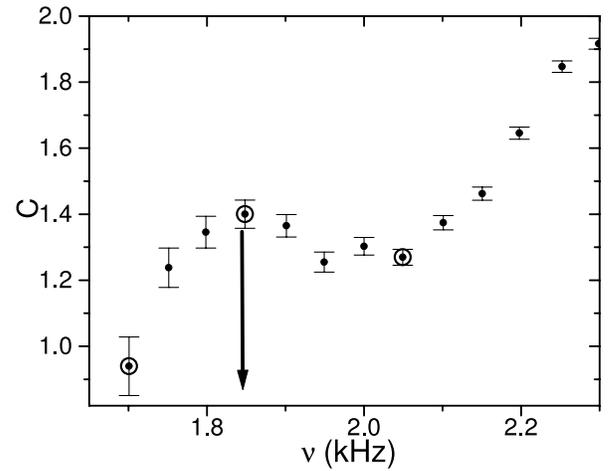
FIG. 3. Coherence factor  $C$  (see text for definition) vs external modulation frequency  $\nu$ . The arrow at  $\nu_{\text{PPS}} \approx 1.84$  kHz indicates the frequency value for which phase slips are maximally coherent. The circles surround the three points for which measurements of  $\Delta(t)$  are reported in Fig. 2.
