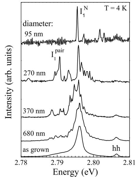
FIG. 1.  $\mu$ -PL spectra of sample A for different mesa diameters under cw excitation with 500 W/cm<sup>2</sup>. All curves are normalized and shifted vertically for a better representation.  $T = 4$  K.
