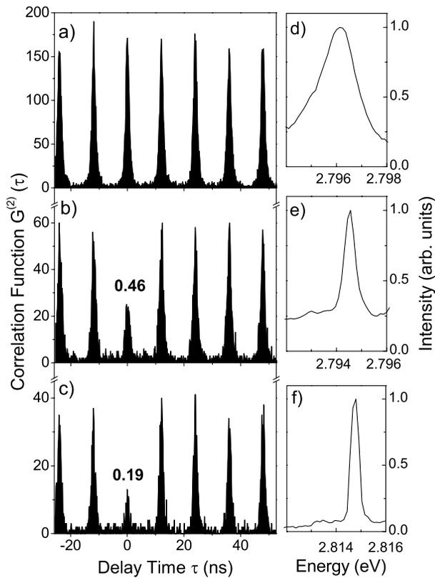
FIG. 3. Measured unnormalized correlation function  $G^{(2)}(\tau)$  in the energy region of the  $I_1^N$  transition for (a) an unstructured part (ensemble average) and for a 95 nm mesa structure of sample A (b) and sample B (c) under pulsed excitation with a Ti:sapphire laser (82 MHz). The corresponding normalized  $\mu$ -PL spectra for traces (a)–(c) are shown in (d)–(f), respectively, recorded with an energy resolution of 500  $\mu$ eV as used for the correlation measurements.  $T = 4$  K.
