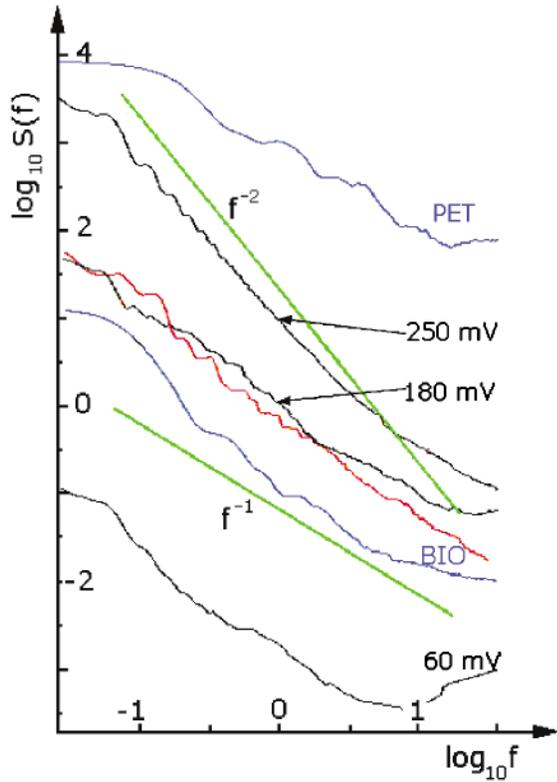
FIG. 2 (color). Smoothed power spectra. Potassium current series data: PET pore excited at different voltages (line labels, black), biological channel BIO (red)—these spectra are in  $(\text{pA})^2/\text{Hz} = 10^{-24} \text{ A}^2 \cdot \text{s}$ ; dwell-time series (blue) for bistable channels: biological (label BIO) and synthetic (label PET)—these spectra are in  $(\text{ms})^2/\text{Hz} = 10^{-6} \text{ s}^3$ .
