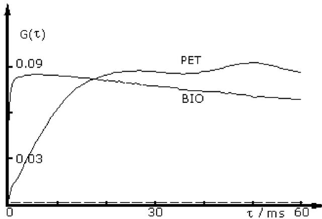
FIG. 4. Non-markovian measure  $G(\tau)$  [Eq. (2)] for bistable potassium current data—biological (BIO) and synthetic PET excited at 180 mV; time range  $T = 60$  ms.  $G(\tau)$  for markovian dichotomous series is shown as a dashed line at the bottom.
