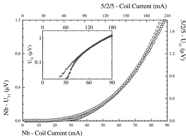
FIG. 3. Scaling of the third harmonic signal for a  $1 \mu\text{m}$ -thick Nb film ( $\square$ ) and a 5/2/5 structure ( $\circ$ ). In the inset, the same scaling is shown in a logarithmic plot.
