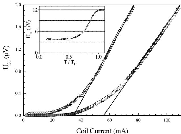
FIG. 2. Third harmonic amplitude as a function of the coil driving current  $I_{\text{coil}}$  for a  $1 \mu\text{m}$ -thick Nb film ( $\square$ ) and a 5/2/5 structure ( $\triangle$ ); linear extrapolation for the calculation of  $I_{\text{coil}}^0$  is reported also. In the inset, the first harmonic transmitted signal  $U_{11}$  is reported as a function of temperature for a 5/2/5 structure.
