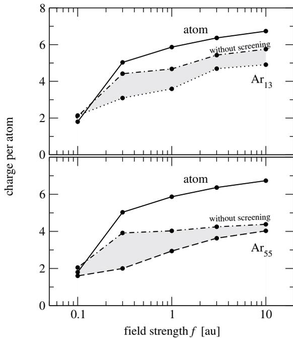
FIG. 4. Average charge per atom for two cluster sizes  $\text{Ar}_{13}$  and  $\text{Ar}_{55}$  produced by an XFEL pulse (same parameters as in Fig. 1) as a function of the field strength  $f$ . Dot-dashed line: Restricted cluster calculation where intracluster screening was precluded.
