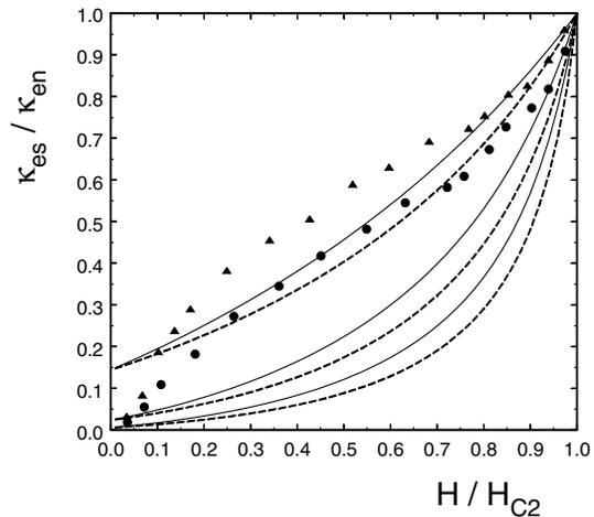
FIG. 2. Electronic thermal conductivity ratio  $\kappa_{es}/\kappa_{en}$  at low temperatures vs  $H/H_{c2}$  for impurity scattering rates  $\delta = 0.1, 0.2$ , and  $0.5$  (from bottom to top). Notation as in Fig. 1: Solid curves for angle  $\theta = \pi/2$ . Dashed curves for the average over  $\theta$ . The dots (triangles) are reduced data from Ref. [6] for  $\text{MgB}_2$  at  $T = 7.94$  K ( $T = 5.13$  K).
