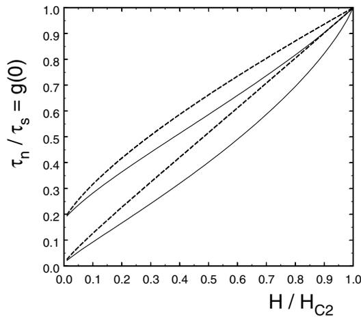
FIG. 4. Ratio  $\tau_n/\tau_s = g(\Omega_0 = 0, H)$  vs  $H/H_{c2}$  for  $\delta = 0.1$  (lower curves) and  $\delta = 0.5$  (upper curves) with the notation of Fig. 3. This quantity determines the reduction of the phonon thermal conductivity at low temperatures due to the increase of scattering by quasiparticles. The solid curves are the average of  $g$  over  $\theta$  corresponding to a spherical Fermi surface and the dashed curves are  $g$  for constant  $\theta = \pi/2$ .
