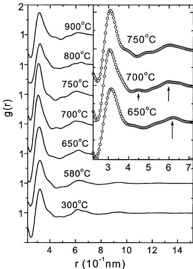
FIG. 3. Patterns of the pair correlation function  $g(r)$  of the melt In-Sn80 at different temperatures. Inset: Magnification of  $g(r)$  from the first peak to the second one at 650, 700, and 750 °C.
