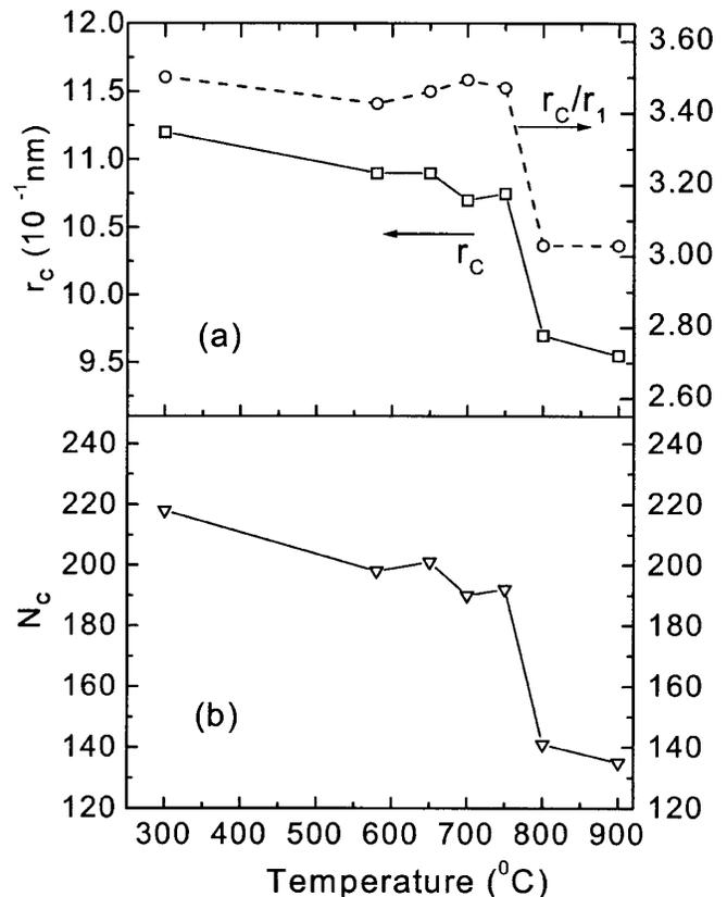
FIG. 2. Both the ordering range and the ordering degree of the melt In-Sn80 decrease abruptly at the end of the structure change. (a) Size of ordering domains  $r_C$  and the ratio (ordering degree)  $r_C/r_1$ ; (b) atom number within the orders  $N_C$ .
