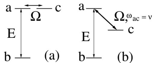
FIG. 3. (a) Static frame. Simplified level structure of level anticrossing: the misalignment component of the magnetic field (providing coupling  $\Omega$  between levels  $a$  and  $c$ ) acts as a driving field in optical schemes [28]. (b) Rotating frame. The coupling static field in the rotating frame acts like an ac field with the frequency equal to transition frequency. The level scheme is resembling the  $\Lambda$  scheme in optics.
