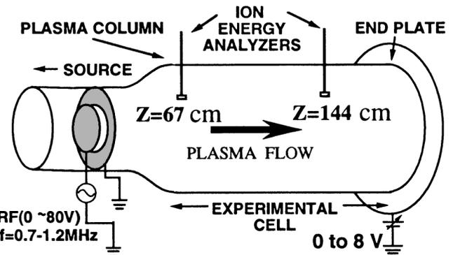
FIG. 1. Schematic of the measurement of transverse ion thermal conductivity via the temperature relaxation scheme.
