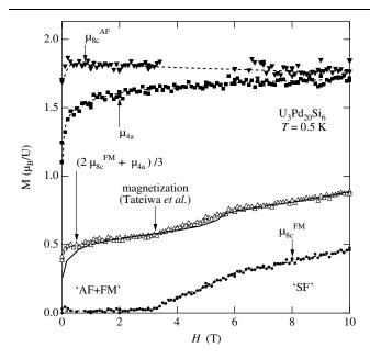
FIG. 6.  $H_{\perp}$  dependence of  $\mu_{8c}^{AF}$ ,  $\mu_{8c}^{FM}$ , and  $\mu_{4a}$ . The broken lines are a visual guide. The total moment  $(\mu_{4a} + 2\mu_{8c}^{FM})/3$  is also plotted and compared with the result of the dc-magnetization measurement [6] denoted by a solid line.
