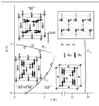
FIG. 1. H-T phase diagram [6] and the magnetic structure in  $U_3Pd_{20}Si_6$ . Inset shows the projection of the uranium atoms on the (110) plane.
