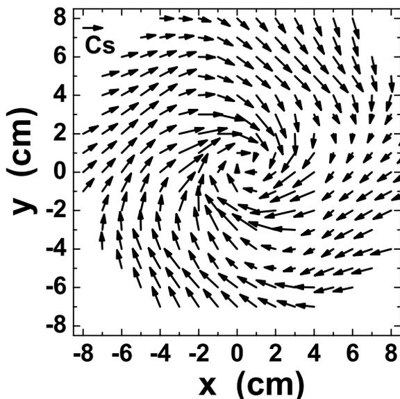
FIG. 2. Two-dimensional velocity field measured at  $z = 110$  cm. The magnitude of arrow corresponding to the ion sound speed is shown at the top left of the figure.
