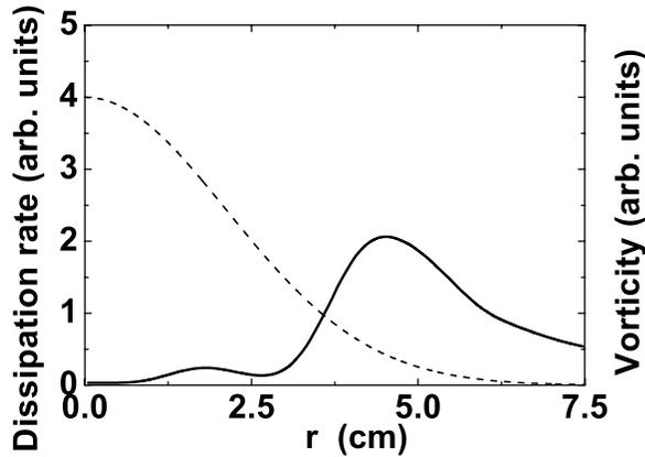
FIG. 5. Dissipation rate as a function of radius. The dashed curve indicates the vorticity distribution.
