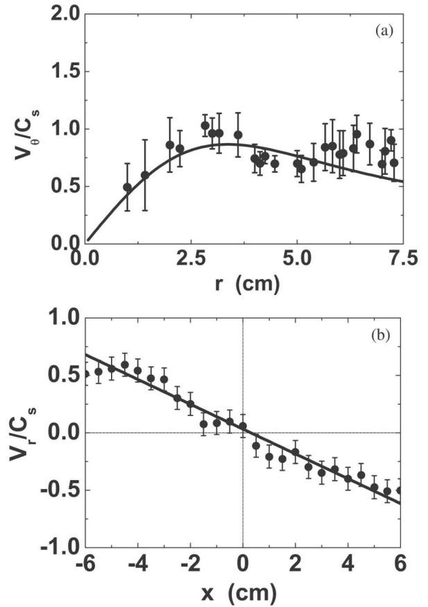
FIG. 4. (a) Azimuthal flow velocity as a function of radius. The solid curve indicates Eq. (2). (b) Radial flow velocity as a function of radius.
