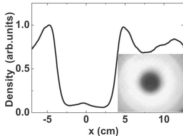
FIG. 1. Radial density profile of the plasma hole ( $z = 110$  cm) and the perspective image taken by a CCD camera located at the end of the chamber.
