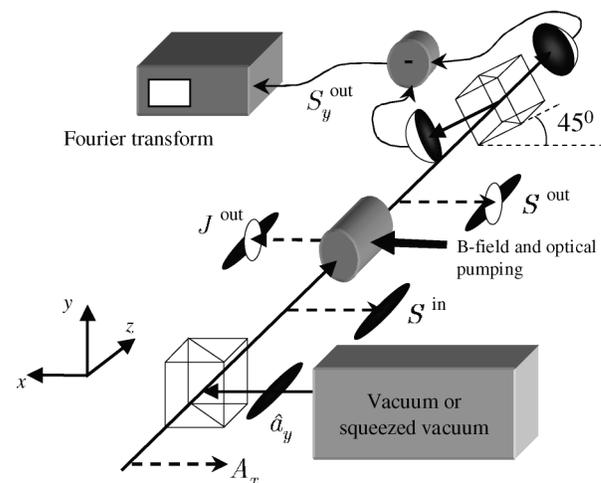
FIG. 1. A vacuum or squeezed vacuum field propagates through the atomic sample, and leaves its trace on the sample. The transmitted light which reads out this trace is analyzed at a polarization state analyzer.
