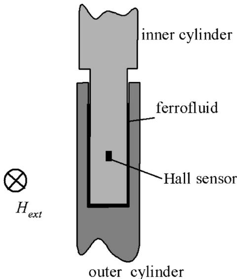
FIG. 2. Schematic sketch of the experimental setup. Details are given in the text.
