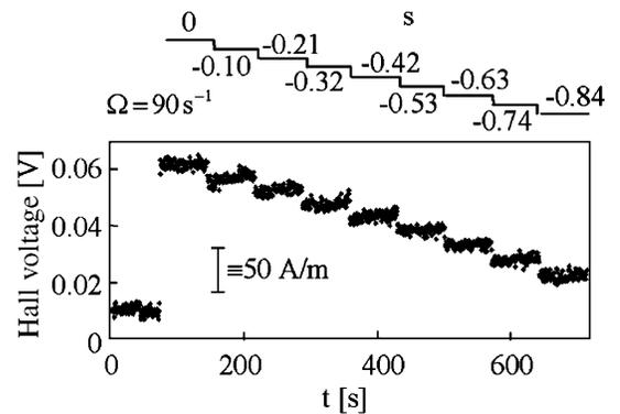
FIG. 3. A typical experiment run: The shear rate was increased by discrete steps in time while keeping the vorticity constant. Simultaneously the voltage signal of the Hall sensor was recorded to detect the  $x$  component of the magnetization.
