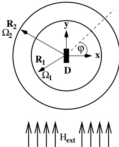
FIG. 1. The ferrofluid is located within a gap between two rotating cylinders with radii  $R_1$  and  $R_2$  rotating, respectively, with the angular velocities  $\Omega_1$  and  $\Omega_2$ . A stationary homogeneous magnetic field  $\mathbf{H}_{\text{ext}}$  is applied in the  $y$  direction. The Hall detector  $D$  in the center records the off-equilibrium component of the magnetization transverse to  $\mathbf{H}_{\text{ext}}$ .
