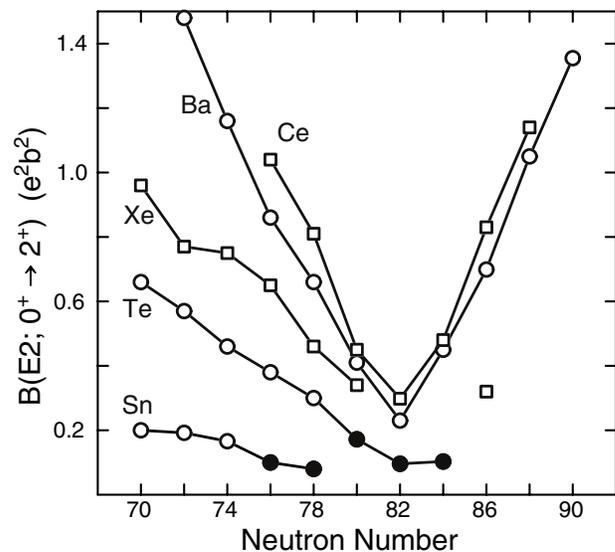
FIG. 2. Values of  $B(E2; 0^+ \rightarrow 2_1^+)$  for even-even Sn, Te, Xe, Ba, and Ce isotopes around neutron number  $N = 82$ . Open symbols are adopted values from Ref. [8], while filled symbols are from the present work (Te) and from Refs. [4,10] (Sn).
