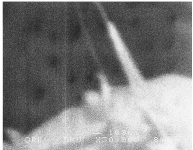
FIG. 1. Scanning electron micrograph showing two grains of Bi/ \text{SiO}_2 nanocomposite. Bi nanowires extend beyond the grain perimeter, and assure electrical contacts between the grains. The wire diameters cannot be estimated from this image, because the nanowires are subject to mechanical vibrations, and very low beam voltages and currents were used to avoid melting the Bi.
