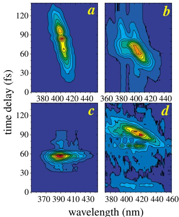
FIG. 2 (color). FROG traces of the probe pulse at different experimental conditions (see text) for rotational excitation in  $\text{H}_2$  and compression.
