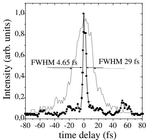
FIG. 4. Self-diffraction autocorrelation traces with (solid line) and without (dotted line) impulsive excitation of  $\text{SF}_6$ . Deconvoluted pulse duration is 3.8 fs (see text).
