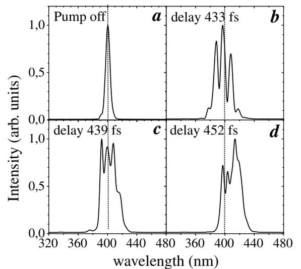
FIG. 1. Probe pulse spectrum in dependence on the delay between the pump and the probe pulses without (a) and with (b), (c), (d) rotational excitation in  $\text{H}_2$ .
