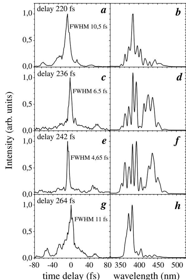
FIG. 3. Self-diffraction autocorrelation traces and corresponding spectra for different delays between the pump and the probe pulses for vibrational excitation in  $\text{SF}_6$ .
