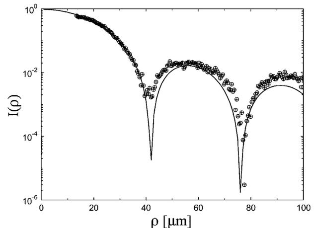
FIG. 2. Radial dependence of intensity in the geometrical focus plane and the corresponding calculation based on the scalar Debye diffraction theory.
