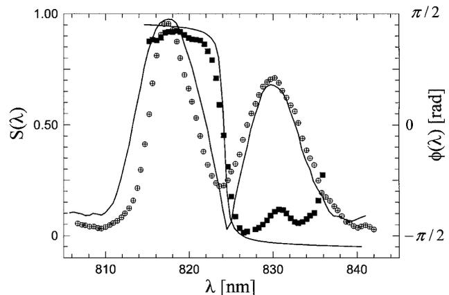
FIG. 4. Optical spectral density and spectral phase modifier measured at  $\rho = 76.2 \mu\text{m}$ . The continuous lines are the results of the Debye theory for the experimental situation.
