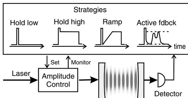
FIG. 1. Experimental setup showing the cavity and the control unit with the different strategies. “Hold low,” “hold high,” and “ramp” are deterministic. In the feedback strategies, the pump power after the initial stopping pulse depends on the motion of the atom, but is bound as indicated by the two dashed lines. The atomic fountain (not shown) injects slow  $^{85}\text{Rb}$  atoms from below into the cavity.
