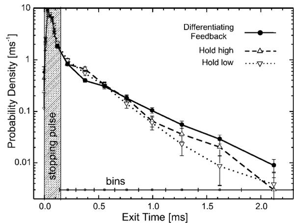
FIG. 3. Histogram of exit times. The width of the histogram bins is shown at the bottom. The hatched area indicates the 0.15 ms long stopping pulse.
