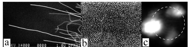
FIG. 1. (a) Scanning electron microscope image of the MWNT sample grown by CVD used in this experiment. (b) TEM image of a MWNT grown by the same method. (c) FE pattern. The bright areas follow approximatively a circle and correspond to one MWNT. The TEDs presented correspond to the bright spot.
