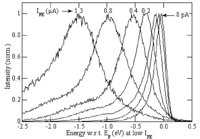
FIG. 2. TEDs for different emission voltages and currents.
