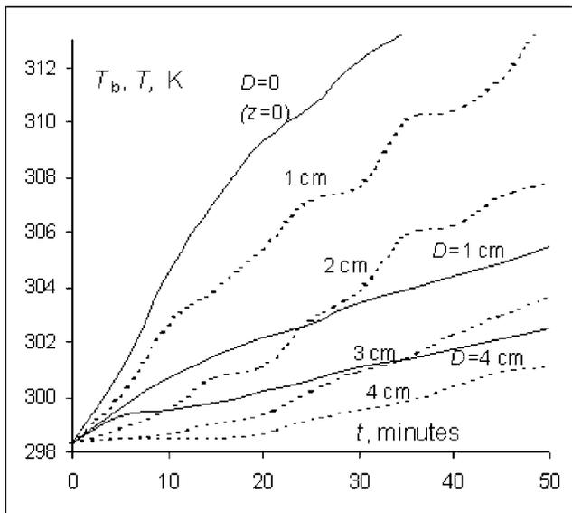
FIG. 4. Measurements of brightness temperature dynamics (solid lines); contact measurements of temperature dynamics at different levels inside water (dashed lines).
