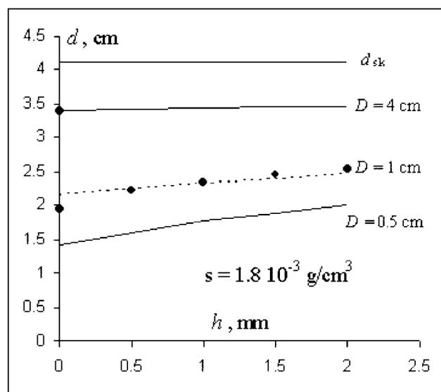
FIG. 3. Effective thickness  $d_{\text{eff}}$  as a function of antenna height for different antenna sizes. Circles correspond to measurements; lines correspond to calculations.
