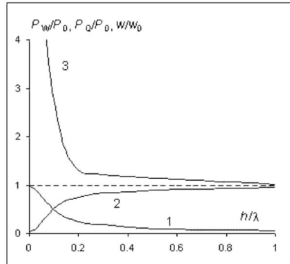
FIG. 1. Normalized power of wave and quasistationary fields as a function of antenna height for  $D/\lambda = 0.01$ : (1)  $P_Q/P_0$ , (2)  $P_W/P_0$ , and (3)  $w/w_0$  according to [1,2].
