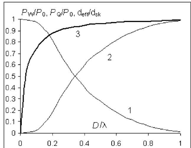
FIG. 2. Normalized power of wave and quasistationary fields versus the antenna aperture size for  $h = 0$ : (1)  $P_Q/P_0$ , (2)  $P_W/P_0$ , and (3)  $d_{\text{eff}}/d_{\text{sk}}$ .
