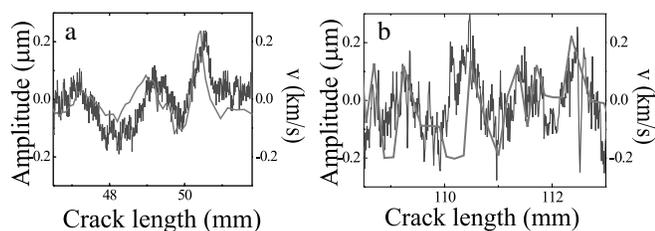
FIG. 2. Comparison, on the  $z = z_{\max}$  plane, of velocity fluctuations (bold line) and the fracture surface height (thin line) generated by FW for (a) FW generated by an external asperity at  $v = 1000$  m/s ( $0.72v_c$ ) and (b) FW generated by microbranching events at  $v = 1500$  m/s ( $1.08v_c$ ). The velocity measurement resolution ( $0.1 \mu\text{sec} \sim 0.05\text{--}0.1$  mm) was not sufficient to capture the fine structure of the surface measurements.
