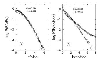
FIG. 3. (a) Force distribution  $P(F/\langle F \rangle)$  obtained by scaling F by the average force  $\langle F \rangle$  of each configuration using the harmonic potential in 3D with N=1024. The solid line is a Gaussian fit to the high-force tail. (b) Same as (a) except F is scaled by  $\langle \langle F \rangle \rangle$  averaged over all configurations.
