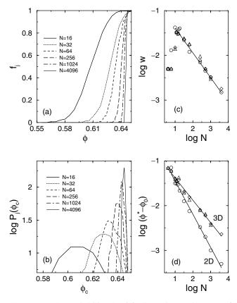
FIG. 2. (a) The probability  $f_j$  of finding a jammed state vs  $\phi$  for  $\alpha=2$  in 3D and several system sizes, N. (b) The probability distribution  $P_j(\phi_c)$  of finding a jamming threshold  $\phi_c$  for systems considered in (a). (c) Full width at half maximum w of  $P_j(\phi_c)$  vs N. (d) The deviation in peak position  $\phi_0$  of  $P_j(\phi_c)$  from its asymptotic value  $\phi^*$  vs N. Data for (c) and (d) are for systems considered in Fig. 1 except  $\alpha=5/2$  in 2D.
