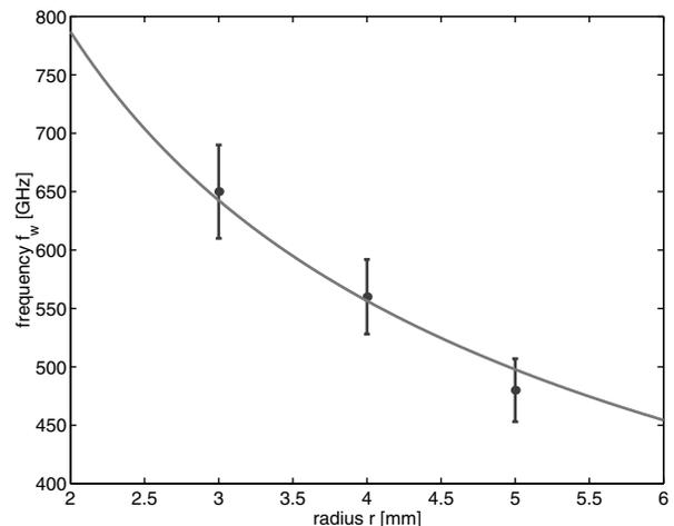
FIG. 4. The frequency of the synchronous mode plotted versus the radius of the beam pipe. The measured frequencies agree within the errors with the  $1/\sqrt{r}$  dependence expected from the dielectric-layer model.
