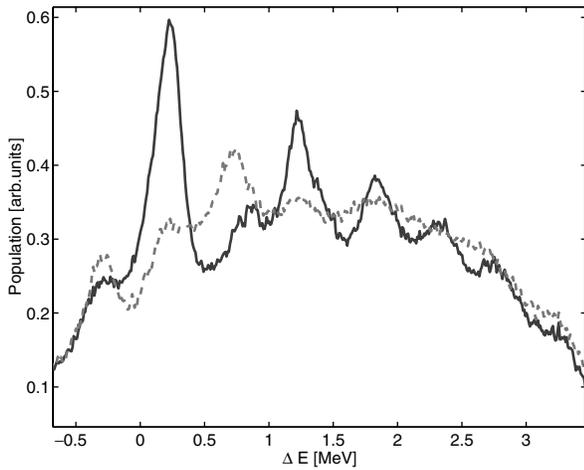
FIG. 3. Energy profile of the tail of a bunch having passed the 4 mm radius test tubes. The dashed curve represents the reference (smooth) pipe, and the solid curve represents the sandblasted pipe. The two pipes are of identical geometry, the only difference is the rms surface roughness of  $1.4 \mu\text{m}$  and  $8.3 \mu\text{m}$ , respectively. The head of the bunch would appear at the left side of the plot but is not visible due to its low energy.
