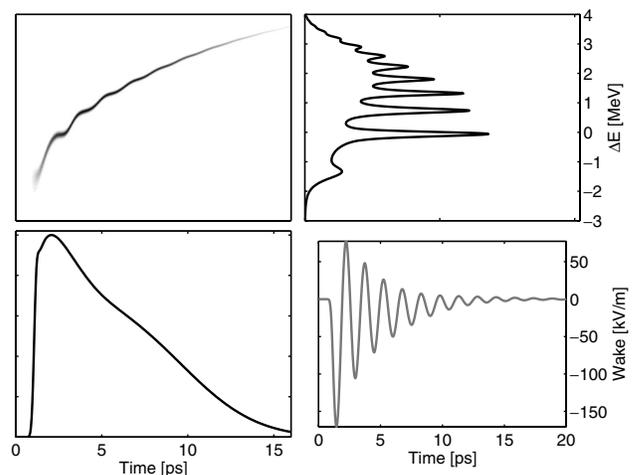
FIG. 2. Simulation of a bunch in longitudinal phase space in the presence of a synchronous mode wake field. The upper left panel shows the bunch in phase space, the lower left shows the projection onto the time axis, and the upper right shows the projection onto the energy axis. The lower right panel shows the harmonic wake field. The periodic energy shift, together with the time-energy correlation, generates the peaks in the energy distribution.
