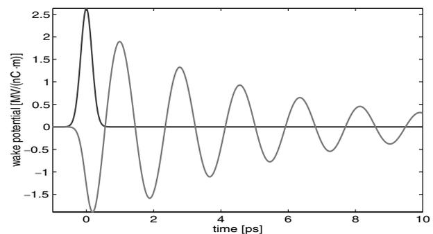
FIG. 1. Longitudinal charge distribution in a Gaussian bunch and the computed wake potential created by a dielectric surface layer [see Eq. (2)]. The bunch head is at the left side. The damping of the periodic wake potential is caused by the finite length and resistivity of the beam pipe. The parameters are  $r = 4 \text{ mm}$ ,  $\delta = 8 \mu\text{m}$ ,  $\varepsilon_{\text{eff}} = 2$ .
