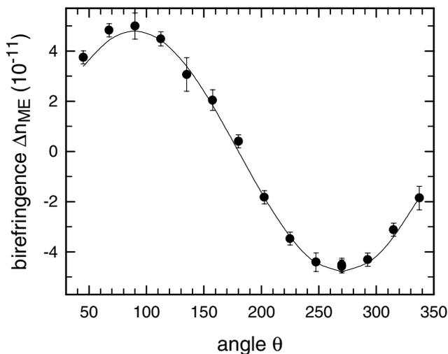
FIG. 4. Angular dependence of the magnetoelectric linear birefringence.  $\Delta n_{ME}$  of “1” as a function of  $\theta$ . A fit to a  $\sin\theta$  dependence is shown. Data were obtained at  $B = 14$  T and  $E = 1.1 \times 10^5$  V/m.
