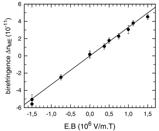
FIG. 3. Magnetolectric linear birefringence.  $\Delta n_{\text{ME}}$  of “1” as function of  $\mathbf{E} \cdot \mathbf{B}$ , with a linear fit to the data.
