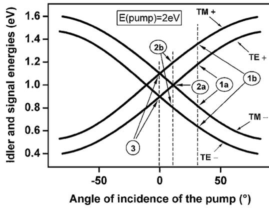
FIG. 3. Tuning curves of counterpropagating PF as a function of the angle of incidence, for an example of pump power of 2 eV. For a given angle of incidence, four photons can be down-converted, since two distinct processes are possible. The positions of processes which are represented in Fig. 1 are indicated.
