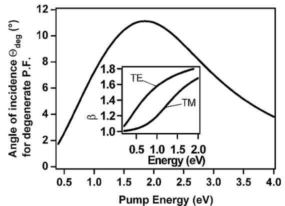
FIG. 2. For a large interval of pump energies, an angle of incidence exists for which degenerate PF is possible. This angle reflects the birefringence of the waveguide, which is maximum for signal and idler photons around 1 eV in our example (see the effective indices of the waveguide in the inset), and thus for a pump at 2 eV.
