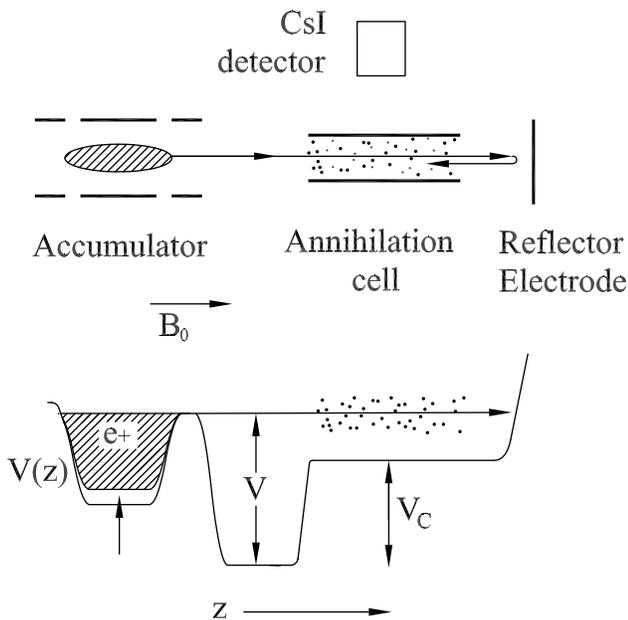
FIG. 1. Schematic diagram of the experiment (above), and corresponding electrical potential  $V(z)$  as a function of position along the magnetic field (below). A cold positron beam is passed through a gas cell. The energy of the beam,  $\varepsilon$ , can be tuned from 50 meV to several electronvolts. To avoid background, the positrons are kept in flight while annihilation events are recorded.
