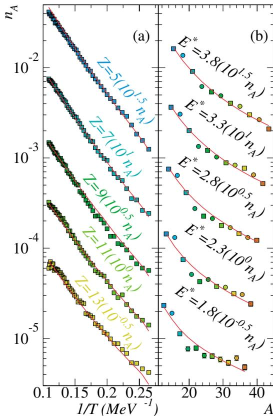
FIG. 1 (color). (a) Arrhenius plots for representative charges, the fragment mass yields versus inverse temperature for the ISiS data. (b) Fragment mass yields for various values of  $E^*$ . Solid curves are from a fit to Fisher's model. See Fig. 2 for symbol definition. Error bars are smaller than the size of the points.
