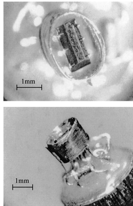
FIG. 1. Sample arrangement for the Knight shift. Upper panel: A top view shows an oval shaped NMR coil and three pairs of electrical contacts on the crystal. Lower panel: A side view also shows a sub-mm diameter pickup coil used to inductively measure  $T_c$  of Pb, and thus the pressure.
