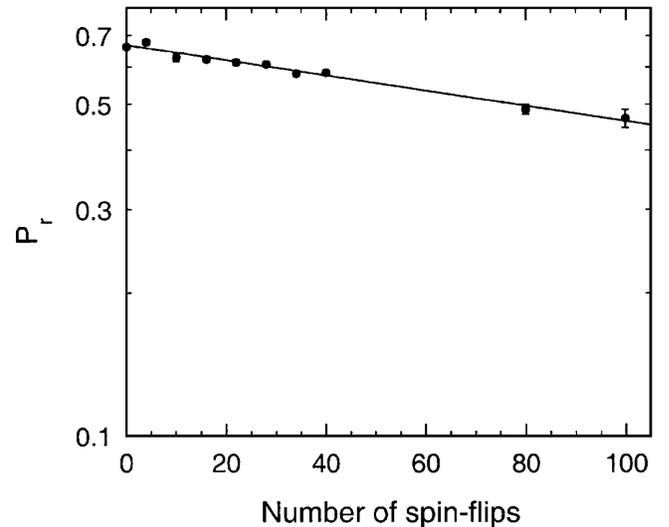
FIG. 6. The measured radial proton polarization at 120 MeV is plotted against the number of spin flips. The rf dipole's frequency ramp time  $\Delta t$  was 100 msec; its frequency range  $\Delta f$  was  $\pm 5$  kHz, and its voltage was 100 V rms corresponding to an  $\int B dl$  of 0.16 Tmm rms. The curve is a fit to the data using Eq. (7).
