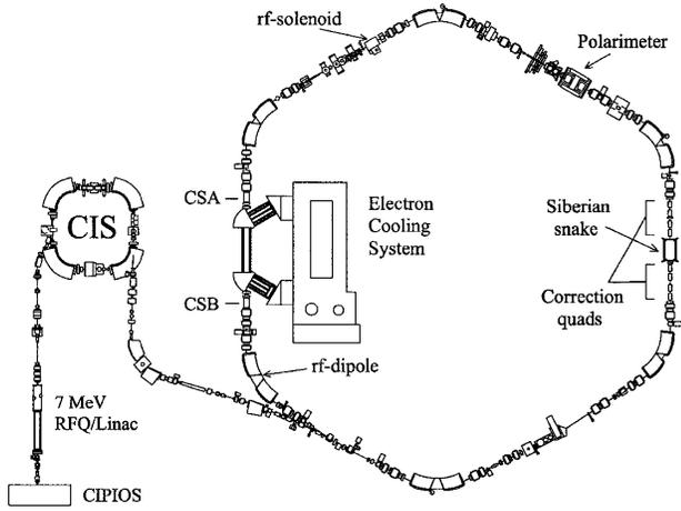
FIG. 1. Layout of the IUCF Cooler Ring with its new Cooler Injector Synchrotron (CIS) and its new CIPIOS polarized ion source. Also shown in the Cooler Ring are the rf dipole, the rf solenoid, the polarimeter, and the Siberian snake.
