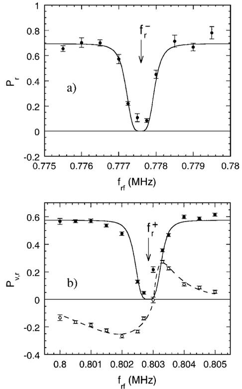
FIG. 3. The measured radial (and vertical) proton polarizations at 120 MeV are plotted against the rf-dipole's fixed frequency for the  $f_r^-$  (a) and  $f_r^+$  (b) resonances. The rf dipole's  $\int B dl$  was 0.10 T mm rms. The solid curves are fits using a second-order Lorentzian. The dashed curve in (b) is a hand-drawn curve to demonstrate the interesting behavior of the vertical polarization when the rf voltage is turned on adiabatically. The arrows show  $f_r^-$  and  $f_r^+$ .
