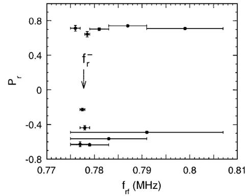
FIG. 2. The measured radial proton polarization at 120 MeV is plotted against the range of each frequency ramp; each frequency ramp's  $\Delta f$  range is shown by a horizontal bar. The rf dipole's  $\int B dl$  was 0.10 T mm rms; its  $\Delta t$  was 1 s. The arrow shows  $f_r^-$ .
