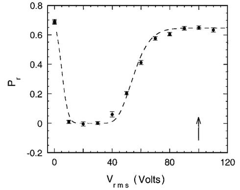
FIG. 5. The measured radial proton polarization at 120 MeV after ten spin flips is plotted against the rms rf-dipole voltage  $V_{rms}$ . The rf dipole's frequency range  $\Delta f$  was  $\pm 5$  kHz, and its ramp time  $\Delta t$  was 100 ms. The dashed curve is a fit to the data using Eq. (6); the arrow shows the 100 V setting used for later studies, corresponding to  $\int B dl = 0.16$  Tmm rms.
