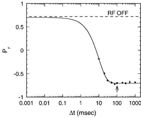
FIG. 4. The measured radial proton polarization at 120 MeV is plotted against the rf-dipole ramp time  $\Delta t$ . The rf dipole's frequency range  $\Delta f$  was  $\pm 5$  kHz, and its  $\int B dl$  was 0.16 Tmm rms. The curve is a fit to the data using Eq. (3). The dashed line shows the polarization with the rf dipole off; the arrow shows the 100 ms setting used for later studies.
