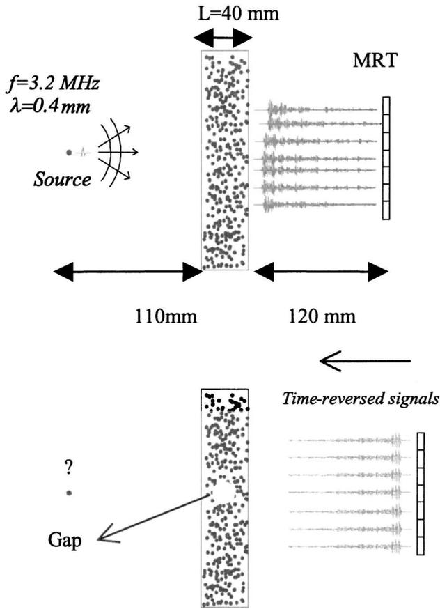
FIG. 1. Top: an ultrasonic source transmits a pulsed wave into a random medium. Bottom: the 128 transmitted signals are recorded on the transducer array and time reversed. At this step, a defect may be introduced in the medium or the temperature can be changed. Then, the time-reversed signals are retransmitted.
