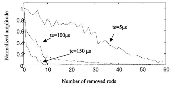
FIG. 4. Peak amplitude versus the number of removed rods for different positions  $t_e$  of the end of the time-reversal window.
