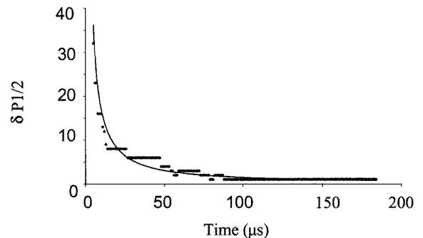
FIG. 5. Time-reversal robustness parameter versus the end time of the time-reversal window.
