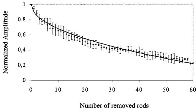
FIG. 3. Peak amplitude versus the number of removed rods. The experiment was carried out five times to obtain the averaged curve. The theoretical prediction based on Eq. (3) is in a continuous line.
