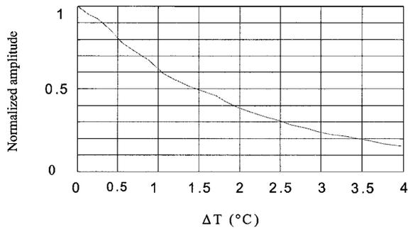
FIG. 6. Peak amplitude as function of a change in temperature.
