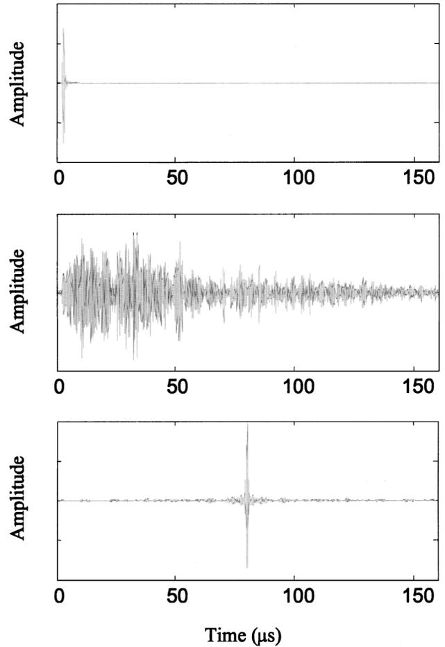
FIG. 2. Signal transmitted in water and received on transducer No. 64 (top). Signal transmitted through the multiple scattering sample and received on transducer No. 64 (middle). Signal  $s(t)$  recorded at the source location after propagation of the time-reversed wave (bottom).
