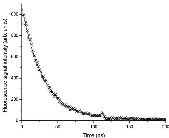
FIG. 3. Typical fluorescence signal from the level at  $49\,737\text{ cm}^{-1}$  in Ce IV showing an exponential fit. The recorded data points are marked as  $\times$  in the figure. The solid curve shows the exponential fit for the LIF signal. The lifetime deduced from the fit was 30.0 ns.
