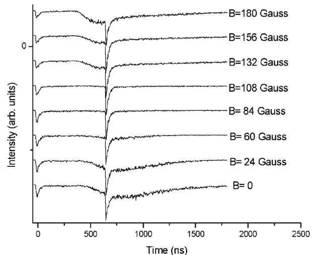
FIG. 2. Time-resolved laser-induced fluorescence signal from the level at  $52\,226\text{ cm}^{-1}$  and background light caused by the laser ablation in different external magnetic fields.  $B = 0$  presents no field over the plasma. A field of about 100 G was observed to eliminate the background.
