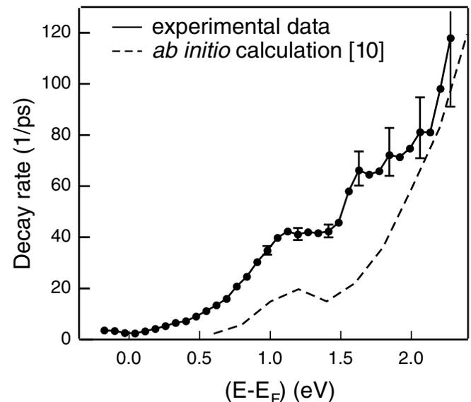
FIG. 2. Energy dependence of decay rates on the pristine HOPG surface. The anomaly near 1.5 eV is indicative of anisotropic QP lifetimes which is also supported by a recent *ab initio* calculation of QP relaxation rates (dashed line) [10].
