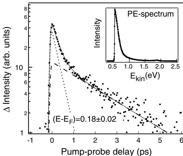
FIG. 1. Cross correlation trace: change of the photoemission intensity in a certain energy interval as a function of the pump-probe time delay. The pump photon energy was 2.3 eV. Fast and slow components of a biexponential fit are indicated by the dotted and dashed lines, respectively. The inset shows a photoelectron spectrum for simultaneous pump-probe excitation.
