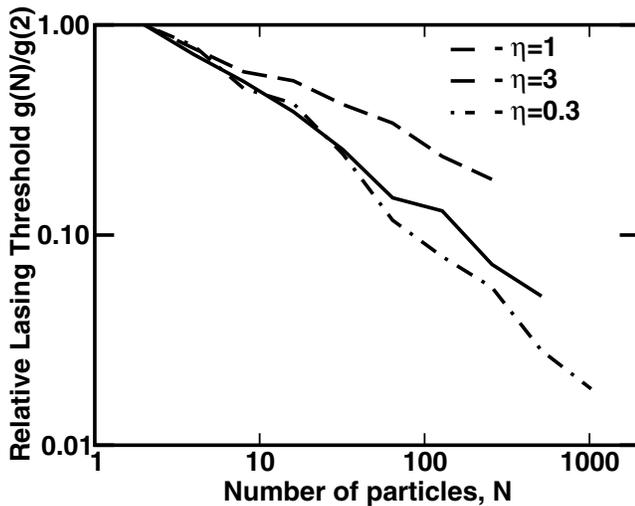
FIG. 1. Dependence of the lasing threshold on the number of particles (sample area).
