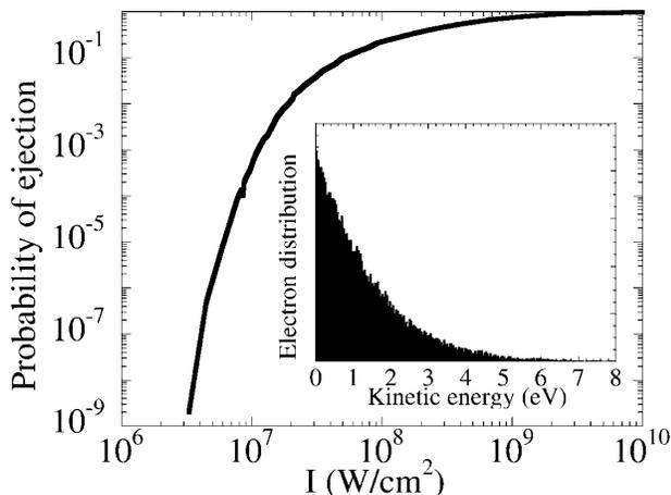
FIG. 1. Simulation of the probability of ejection of an electron as a function of laser intensity. Inset: electron kinetic energy (eV) distribution for  $I = 5 \text{ MW/cm}^2$ .
