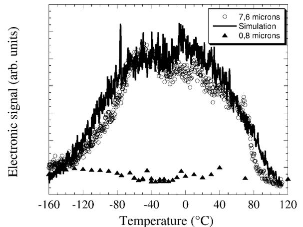
FIG. 2. Electronic signal as a function of the sample temperature (arbitrary units) ( $\bullet$ ): experiment at  $7.6 \mu\text{m}$ ; —: Monte Carlo simulation at  $7.6 \mu\text{m}$ ,  $5 \text{ MW/cm}^2$ ,  $2 \text{ ps}$  pulse duration; ( $\blacktriangle$ ): experiment at  $800 \text{ nm}$  using a Ti:sapphire laser.
