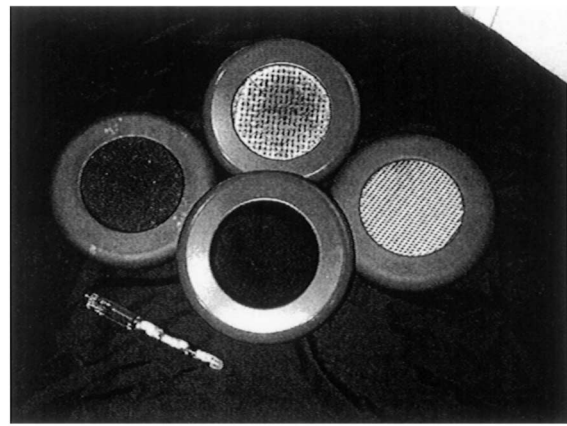
FIG. 7. Photograph of a sampling of cathode types tested at AFRL in identical bushing rings (courtesy of D.A. Shiffler). Top: cesium iodide-coated carbon tufts. Right: metal finger stock on ceramic shutters. Bottom: polymer velvet. Left: cesium iodide-coated carbon fibers.
